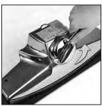
7 Turn the Belt Lifter counterclockwise until the red arrows line up. The belt should catch on the hook inside the nozzle. Reattach the Power Nozzle to the unit.
