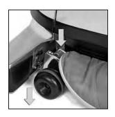
$3\,$  Put Tech Drive® power assist in neutral. Lower the Power Nozzle and vacuum the floor.
