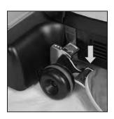
6 Press the Toe-Touch Control Upper Pedal repeatedly until the Miracle Shine Mop contacts the floor. Immediately move the cleaner over the sprayed area to spread the Miracle Shine in an even layer. For best results, only go over the area with one or two quick passes; additional passes of the Kirby system may cause streaks. Spray additional solution as needed.
