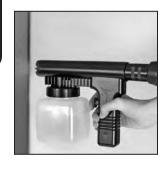
${f 3}$  Squeeze the trigger fully and use slow, sweeping motions when spraying.
