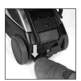
A Make sure Tech Drive® power assist is in neutral and turn the cleaner on.
