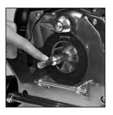
Keep Motor Shaft free from lint, hair and debris built-up.
