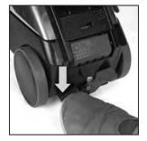
Put Tech Drive power assist in neutral by pressing down on the side of the pedal marked N for neutral. This makes it easier to push or pull the unit when the motor is turned off.
