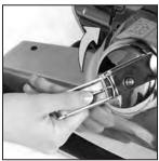
8 Turn the Belt Lifter clockwise until the green arrows line up.
